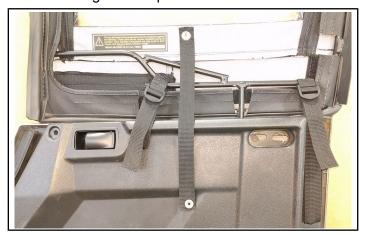
7. Install pull strap ② to upper door ② by wrapping each end of strap around door frame, then snapping into place as shown.
