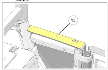
b. Carefully drill 1/2 inch (13 mm) hole at each marked location.
