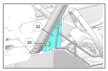
b. Install outboard trim ② to inboard trim ② using two screws ③.
