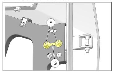
b. Loosely install front post bracket ® to inner surface of door frame using two retained hinge screws F and double-washer G.
