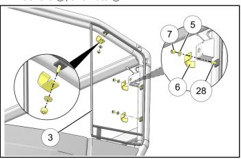
3. Loosely install bolster panel ③ post to vehicle frame using bolster panel bracket ⑧, screw ④, washer ⑤, and nut ⑦.
