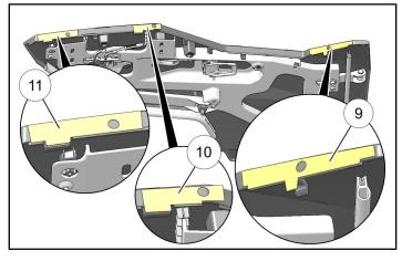
e. Carefully drill 1/2 inch (13 mm) hole at each marked location.
