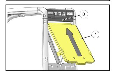
4. While keeping upper edge of panel ① on FORWARD side of ROPS cross member ®, tilt lower edge of panel forward. Slip both panel brackets ② over cab cross member ®, then lower panel until brackets are fully engaged. Ensure panel is centered from right to left.
