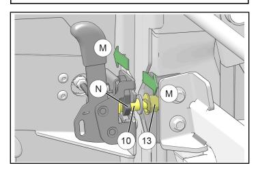
11. Torque striker screws (4) to specification.
