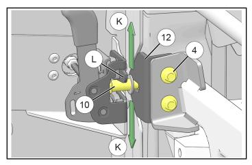
b. **DEPTH** (M): As required to achieve desired fairing between door assembly (1) and ROPS/chassis structure. To adjust, loosen nut (3), slide striker pin (10) inboard or outboard as required, then retighten nut.
