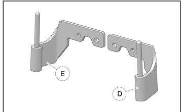
c. Loosely install lower LH chassis-side hinge ① to chassis fitting using two screws ④.
