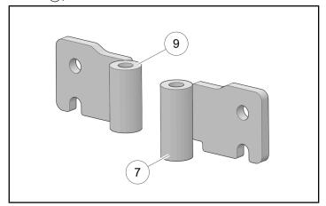
h. Loosely install spacer ® and lower LH chassis-side hinge ⑨ to B-pillar fitting using two screws ④.
