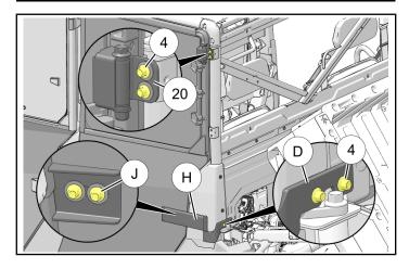
• IF PERIMETER GAP IS UNEVEN: Loosen two lower DOOR-SIDE hinge screws ① (interior of door), center door in opening using slotted fastener openings, then re-tighten same screws.
