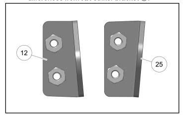
b. Install striker pin (1) and washer (1) to LH striker bracket (1) using nut (3). Center pin in slot, then tighten nut.
