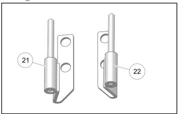
b. Loosely install upper LH chassis-side hinge ② to B-pillar fitting using two each screws ④ and washers ®. Ensure cupped-side of washer is towards hinge.
