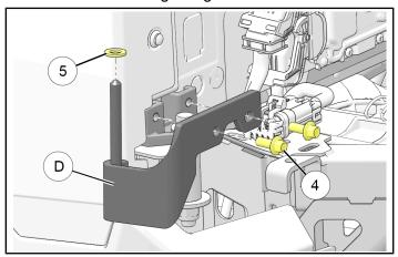
d. Install nylon washer 5 to hinge pin.
