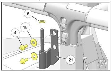
c. Install nylon washer 5 to hinge pin.
