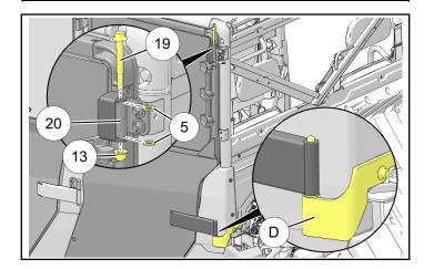
7. With upper and lower chassis-side hinge screws slightly loose, close door.
