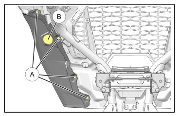
b. Locate center of circular area (B), then drill 1/8 inch (3 mm) pilot hole forward through panel from BACK to FRONT.
