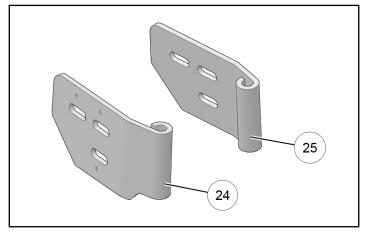
Install upper LH door-side hinge A to LH rear door
