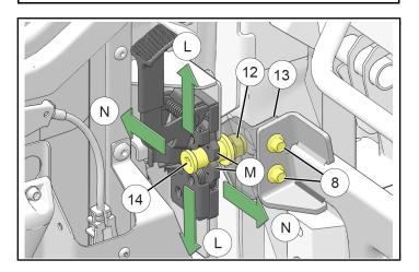
2. Torque striker screws (8) to specification.
