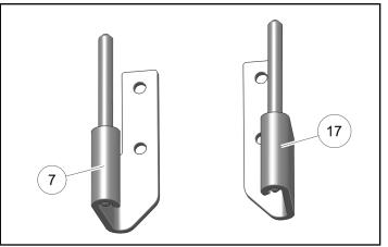
Install upper LH chassis-side hinge ⑦ to B-pillar fitting using two screws ⑧. Partially tighten screws (but still loose enough to allow hinge adjustment). Install nylon washer ⑨ to hinge pin.
