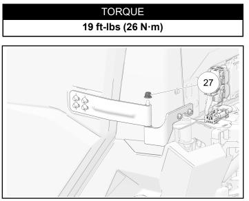
Install limiter strap retaining post to ROPS diagonal support using screw ④, spacer ⑤, and nut ⑥. Torque to specification, then secure strap
