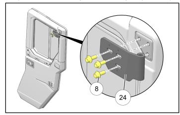
Install lower door-side hinge 3 to LH rear door 1 using four screws (8). Partially tighten screws (but still loose enough to allow hinge adjustment).
