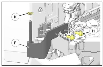
Install upper LH chassis-side hinge (1) to C-pillar fitting using two screws (1) and nut plate (1). Partially tighten screws (but still loose enough to allow hinge adjustment). Install nylon washer (1) to hinge pin.
