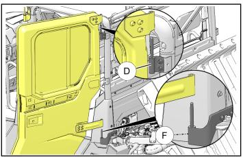
Close and push door inwards while centering door in ROPS/chassis opening, then tighten all screws
