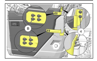
11. Torque all four chassis-side hinge screws ④ and all eight door-side hinge screws ® to specification.
