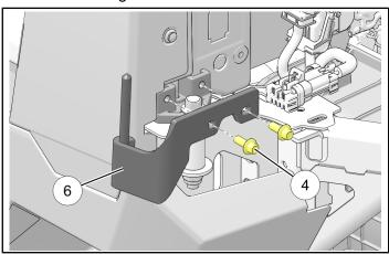
4. Install nylon washer 3 on hinge 6.
