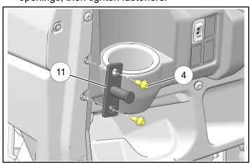
13. Open door latch (to properly position pawls), then slowly close door and observe engagement of striker pin © into door latch D.
