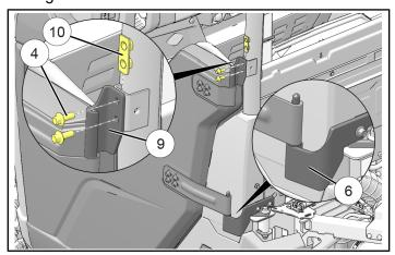
10. Slightly loosen all eight DOOR-SIDE hinge screws ®, then close door. Push door inwards while centering door in ROPS/chassis opening, then tighten screws.
