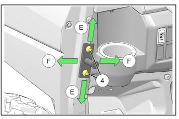
14. Torque striker screws 4 to specification.
