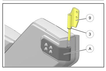
9. Install LH door assembly ① to vehicle by first inserting door onto lower chassis-side hinge ⑥, then install upper chassis-side hinge ⑨ to ROPS bracket using two screws ④ and nut plate ⑩. Tighten screws.
