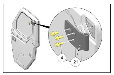
c. Loosely install upper left door hinge (2) to left door ① with three screws ④.
