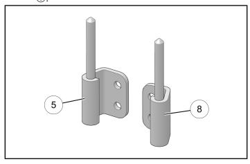
c. Loosely install upper left chassis-side hinge (5) using two screws (4) and nut plate (6).
