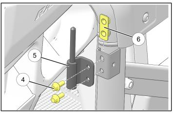
d. Install lower LH chassis-side hinge ⑦ using two screws ④. Loosely tighten screws.
