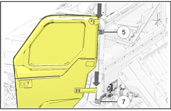
b. Close and push door inward while centering door in ROPS/chassis opening, then loosely tighten all screws ④.
