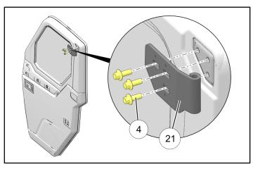
c. Loosely install upper left door hinge ② to left door ① with three screws ④.
