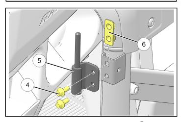
d. Install lower LH chassis-side hinge ① using two screws ④. Loosely tighten screws.
