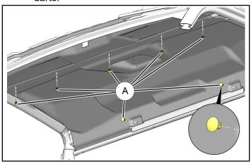
c. If overhead light is installed against liner, remove it. Otherwise, remove two each screws
