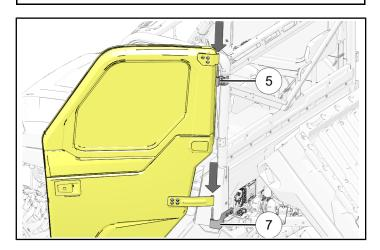
b. Close and push door inward while centering door in ROPS/chassis opening, then loosely tighten all screws 4.
