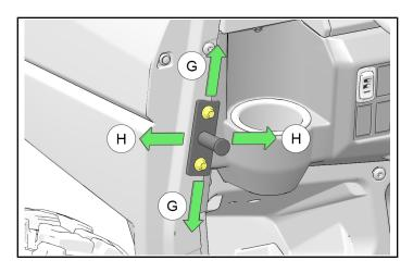
2. Torque striker screws 4 to specification.
