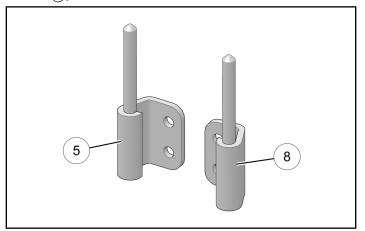
c. Loosely install upper left chassis-side hinge (5) using two screws (4) and nut plate (6).
