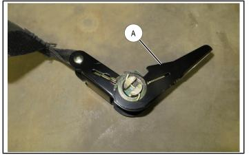
b. Thread RH strap through loop on end of center strap.
