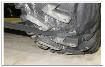
e. Tension strap sufficiently to prevent it from slipping above tire lugs during transport, then fully close ratchet lever (A).
