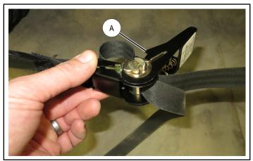
d. Operate ratchet mechanism until slack is removed, then EXAMINE ALL FOUR TIRES to ensure strap is positioned BELOW lower tire lugs as shown. Adjust as necessary.
