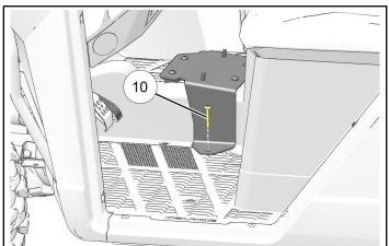
4. Temporarily install RH front side of floor bracket ① to vehicle using retained push pin rivet ⑧.
