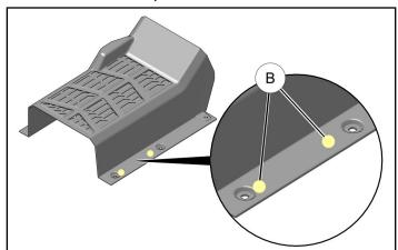
3. Drill 5/16 inch (8 mm) hole through LH floor liner at dimpled location ©.
