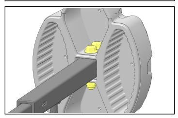
5. Install two V-clamps ① to cap ⑤ and inside tube ⑥ using two each 60 mm screws ④ and nuts ⑤.
