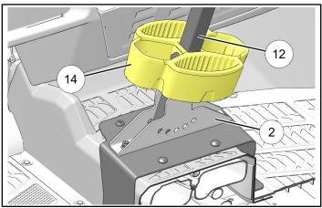
b. Install 60 mm screw ① through UPPER holes in pivot bracket ② and outside tube ⑫. Secure with nut ⑤, but do not tighten at this time.
