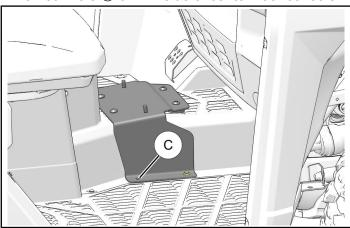
6. Remove floor bracket ① by removing screw ⑩ from LH side of bracket, and push pin rivet ⑧ from RH side of bracket. Retain screw and rivet.
