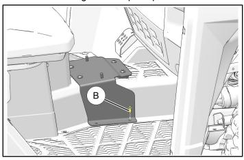
5. Using floor bracket ① as template, mark location of rear hole © on RH side of center floor console.
