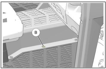
3. Temporarily install LH side of floor bracket 1 to vehicle using screw 0.
