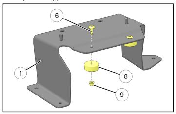
3. Install rubber bumper ① to REAR end of floor bracket ① by pushing button-end up through hole. Repeat for opposite side.
