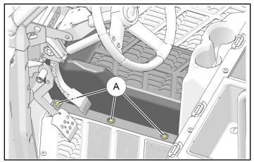
2. Drill two 5/16 inch (8 mm) holes through RH side of console at dimpled locations (8).
