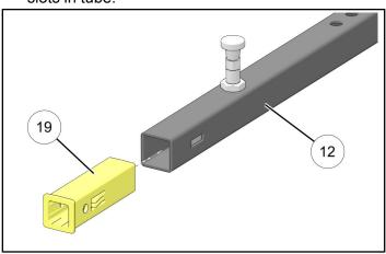
2. Insert inside tube ® into lower end of outside tube
