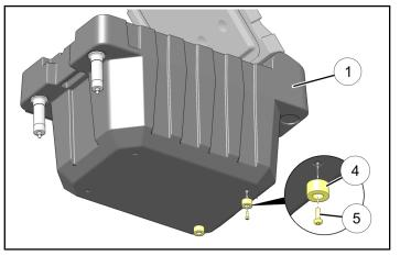
4. Ensure all expansion anchors ② are unlocked, then install storage box ① into bed until anchors are fully seated. Depress levers to lock in place.
