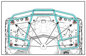
4. Place center section of rack ② in the location shown. Use contours on rear storage bin cover to align center rack section evenly. Once aligned, use a suitable marker or scribe to mark the location of the mounting holes ®.
