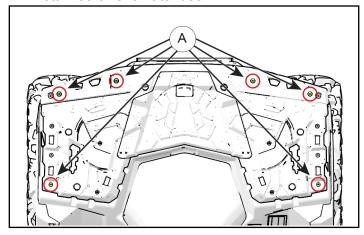
3. Place rack on rear platform, align mounting holes and fasten using the screws (A) removed in the previous step.
