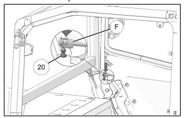
10. Install upper left B-pillar trim ② using two each brackets ③ and screws ⑥. Do not overtighten screws.
