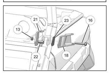
5. Install ball fitting ② to left strut bracket ② using nut ③. Tighten nut.
