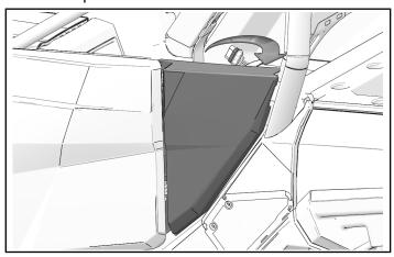
3. Remove three screws and nut from bolster panel frame.
