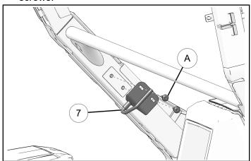
14. Check alignment of front door with B-pillar trim. Adjust front door as needed.
