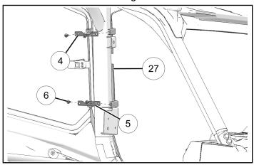
13. Install striker bracket ① to chassis using two retained screws ⓐ. Center bracket, then tighten screws.
