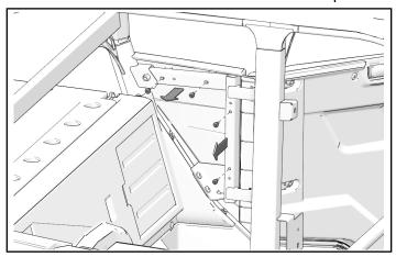
Rotate rear of bolster panel outward and remove bolster panel.
