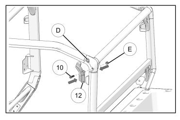
4. Install lower left chassis-side hinge ® and left strut bracket ② to ROPS mounting bracket using 65 mm hex flange bolt ⑥, spacer ②, and nut ③. Torque to specification.
