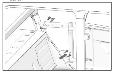
4. Remove bolster panel frame and rear door.
