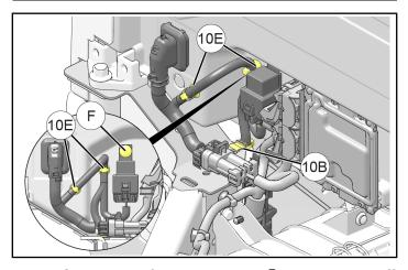
g. Secure rear firewall harness 0 to rear close-off panel using two routing clips 10E, nail clip F, and edge clip 10B.
