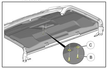
iv. Carefully pull left and right edges of liner from between ROPS and roof seal, then remove rear edge of liner from roof support channel (D).
