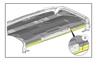
Install terminal block ① to roof using four screws
