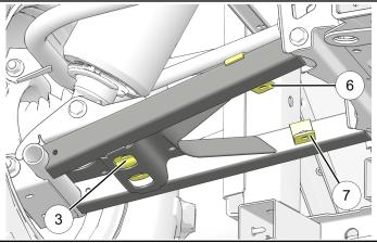
3. Install LH a-arm guard ① to previously installed clamps using four each screws ⑤ and washers ④.
