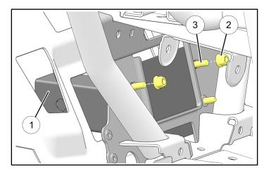
6. Torque all four screws to specification.
