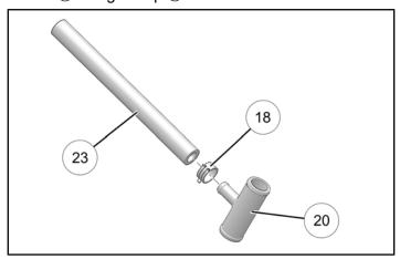
b. Slip second clamp ® over opposite end of hose ③, then install hose to 1/2 inch hose fitting ⊕. Do not clamp hose to fitting at this time to allow hose assembly to rotate into proper position.
