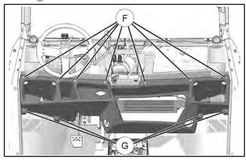
d. Position vent body (with attached duct) at dash opening, then thread vent outlet back onto vent body. Repeat for opposite side.
