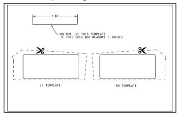
3. Tape each template to the underside of the upper dash, as shown.
