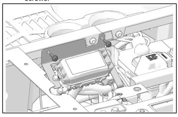
b. Remove and keep fuse box bracket.
