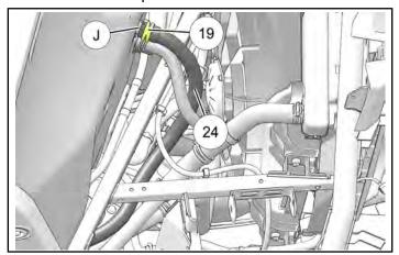
b. Route opposite end (smaller bend radius) of hose @ downward and rearward into center console following existing coolant lines.
