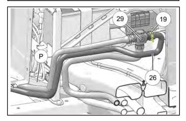
b. Route opposite end of hose (a) across top of air intake duct, down seat structure, then rearward along OUTSIDE of vehicle frame (P) towards oil cooler outlet (1).
