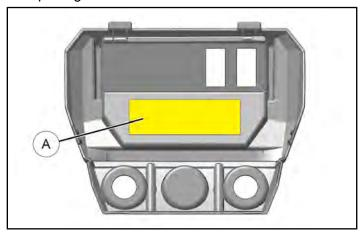
2. Orient switch panel ② so blower control is on LH side and temperature control is on RH side, then install into opening until tabs lock in place.
