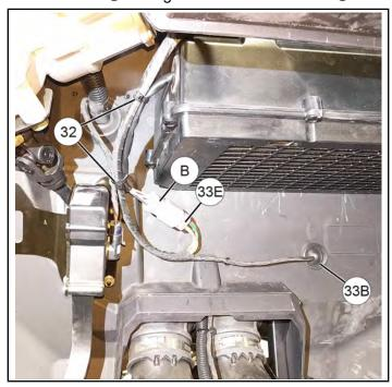
6. Route 3-way valve connector 33D forward through firewall hole © drilled in previous section, **INSTALL HEATER CORE**, Step 4c, then install grommet 33B in hole.
