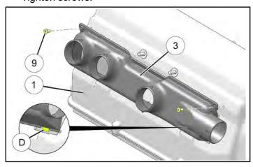
3. Install RH duct assembly ③ to outlet on RH end of manifold ③ until duct contacts stop on manifold. Secure to manifold using cable tie ④.
