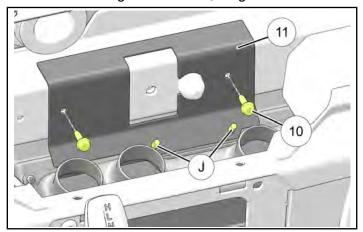
7. Secure heater core upper studs ① to core mounting bracket ⑪ using two nuts ⑫. Tighten nuts.
