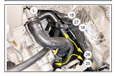
7. Remove hose pinch-off pliers near oil cooler outlet ① and pinch-off pliers on hose ② between hose fitting ④ and tee fitting ② (see Step 3).
