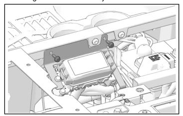
f. Join 3-way valve connector 33D on heater harness 33 to 3-way valve assembly 29.
