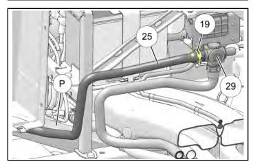
e. Route opposite end of hose ② across top of air intake duct, down seat structure, then rearward along OUTSIDE of vehicle frame ② to water pump inlet ④.
