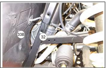
8. Continue routing connector 33D rearward through tunnel along battery cables.
