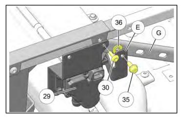
c. Join 3-way valve connector 33D on heater harness 33 to 3-way valve assembly 29.
