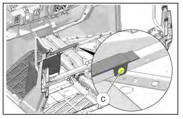
b. Install valve mount bracket (E) (part of 3-way valve assembly (29)) to seat support structure using screw (30), screw (35), and washer (36). Tighten screws.
