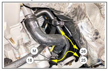
6. Install HOT SUPPLY heater hose between 3-way valve and engine
