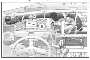
3. Install duct assembly ④ to THIRD outlet on manifold ③ until duct contacts stop on manifold. Secure duct to manifold using cable tie ②.
