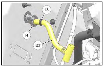
c. Hold tee fitting @ against existing cold hose, rotating new hose ② on fitting ① as required to relieve twist.
