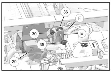
e. Install fuse bracket with two retained screws. Tighten screws until fully seated.
