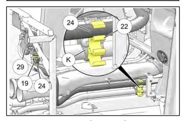
c. Attach routing clip ② to hose ④ using its UPPER (largest) opening, then install routing clip and hose to existing coolant line bracket 𝔾 at front end of center console.
