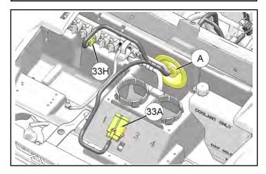
2. Drill out one accessory plug (1/4 inch / 6 mm) on under-hood liner, forward of air intake ducts, then install relay/fuse block 33A using attached fir tree clip.
