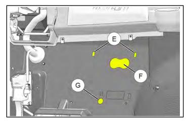
5. Lift heater core assembly ① into position beneath dash, inserting two front studs ④ through vertical slots ⓒ in firewall. Loosely install core to firewall using two each washers ⑥ and nuts ⑰.
