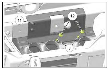
8. Tighten two firewall nuts ① installed in Step 5 of this section.
