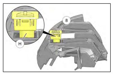
d. Holding upper dash in position, push LH defroster duct ⑤ up through dash. Install rectangular vent ⑧, secure vent to duct using cable tie ⑩, THEN snap vent into dash opening.
