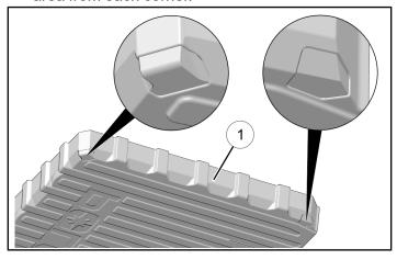
2. Place mat ① into cargo bed. Make sure the mat is fully seated at each corner. If difficulty is encountered with mat installation, remove mat, trim corner opening(s) as required, then reinstall.
