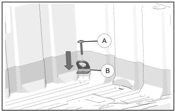
14. If equipped, loosely install the AUX box cover with four retained screws over the bed mat.
