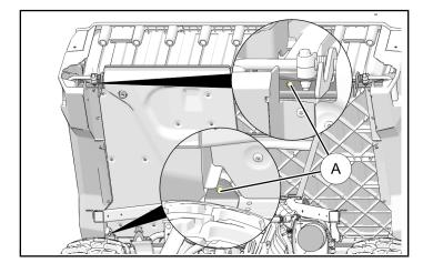
7. Insert ice pick (or equivalent) up through each support structure screw hole to mark hole location on mat.
