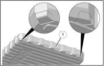
Place mat ① into bed, ensuring mat is fully seated at each corner. If difficulty is encountered with mat installation, remove mat, trim corner opening(s) as required, then reinstall.
