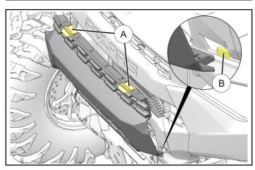
c. Remove upper dash cupholder by removing two push pin rivets ©, then sliding cupholder rearward. Retain rivets.
