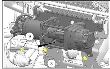
d. Torque screws (8) and nuts (8) to specification.
