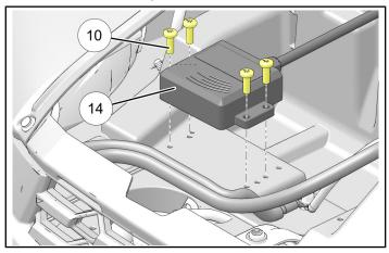
Route wireless receiver connectors 14B and 14C rearward through firewall grommet into upper dash compartment. iii. Locate UNUSED 4-pin main vehicle harness breakout connector (M) in cavity where cupholder was removed in Step 3c. Remove cap from connector, then join to mating wireless receiver connector 14B.
