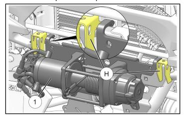
b. At UPPER fastener holes loosely install two screws ® REARWARD through winch into vehicle front support structure.
