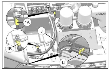
c. Join **RED** 45 degree ring terminal 1A to terminal block battery positive (+). Torque nut to specification, then install boot.
