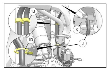
b. Secure terminal block cables ① to under-hood liner using upper routing clip 1J.
