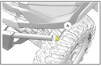
Loosely install threaded mount ⑦ to tapered fitting on LH upper bumper ① using screw ⑧. Screw should engage only a few threads of threaded mount.
