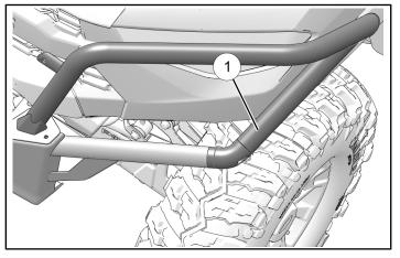
5. Loosely install LH upper bumper ① to existing lower bumper using two screws ⑤ and backing plate ⑥.
