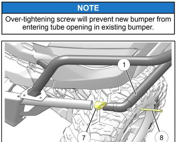
4. Fully insert threaded mount ⑦ and tapered fitting on LH upper bumper ① into existing bumper. Do not tighten screw at this time.
