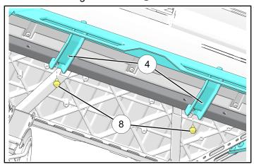
7. Torque all screws ① and ⑧ to specification.
