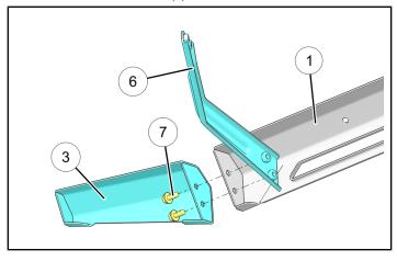
4. Loosely install center support 4 to center bumper 1 using screw 7. Repeat for opposite side.
