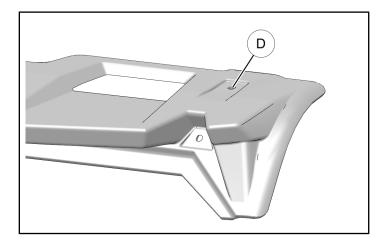
c. Remove and discard clip nut © from UPPER REAR side of ROPS visor bracket. Repeat for RH side.
