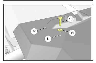
ii. Loosely install front of roof to ROPS using screw ® and washer ® inserted down through roof, spacer ②, and ROPS visor bracket.
