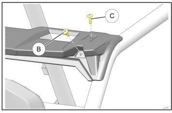
e. Reinstall two retained screws ® through LOWER FRONT visor holes into ROPS as shown in previous step. Torque to specification.
