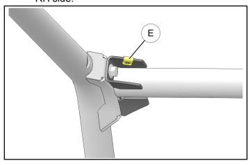
d. Lay visor on ROPS, then temporarily reinsert two retained screws © through UPPER REAR visor holes into ROPS visor brackets.
