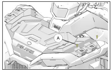
Install modular rack extender ① using screws (A) on front rack as shown. Tighten screws to specification.
