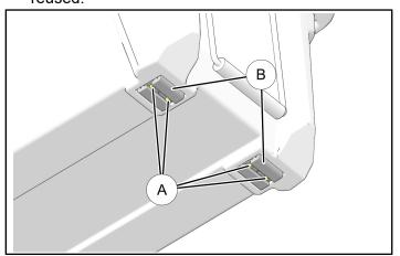
3. Install frame ① to bottom of cooler using two retained pads ® four washers ⑦ and four new screws ⑥. Do not overtighten screws.
