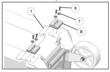
4. Install frame ① to end of cooler using two screws⑤. Do not overtighten screws.
