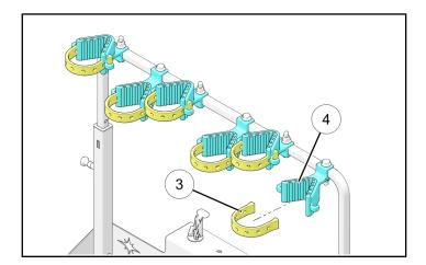
6. Ensure all LOCK & RIDE® expansion anchors ® are unlocked, then install gun rack assembly into bed as shown until anchors are fully seated. Depress levers to lock in place.
