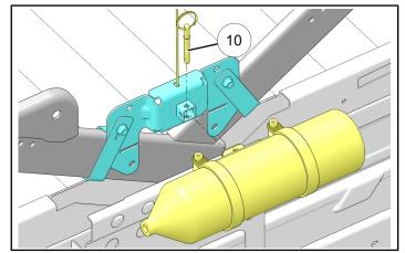
6. Test operation of bottle assembly by removing release pin <sup>(1)</sup>. Adjust location as required to ensure unrestricted access to bottle and freedom of release mechanism.
