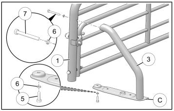
4. Install two LOCK & RIDE® expansion anchors ④ to LH support ③. Repeat for RH support ④.
