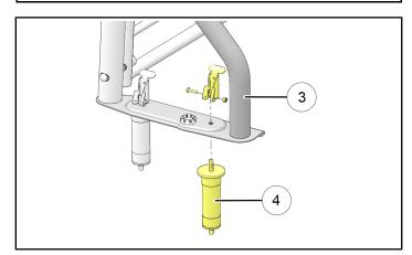
5. Ensure all expansion anchors ④ are unlocked, then install frame ① into bed until anchors are fully seated. Depress levers to lock in place.
