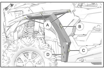
3. Install new LH fender ① using retained screws A
