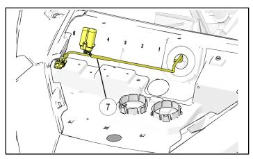
b. Drill out one accessory plug (1/4 inch / 6 mm) on under-hood liner, then install relay/fuse block (H) using attached fir tree clip.
