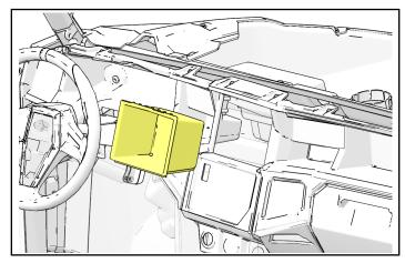
iii. Using fingers, remove center control panel by disengaging four spring clips ①.
