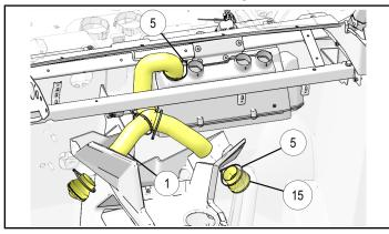
b. Duct ②: Route from heater core to LH outboard dash and LH defrost. Secure duct at heater core with cable tie ⑤.
