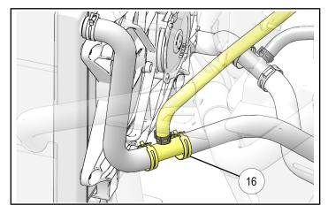
vii. Install hose assembly ① to "IN" coolant line fitting ②. Ensure hose is fully seated, then secure with 20 mm hose clamp ①.
