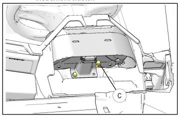
ii. Using fingers, remove center storage box by pressing top edge of box down, disengaging box locking tabs from main dash panel. Tip box out of dash and remove.
