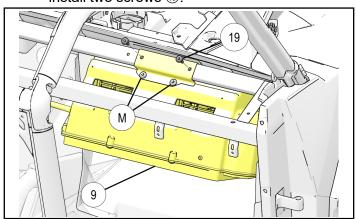
e. Secure front of heater core to firewall using three each screws ② and washers ③. Tighten screws.
