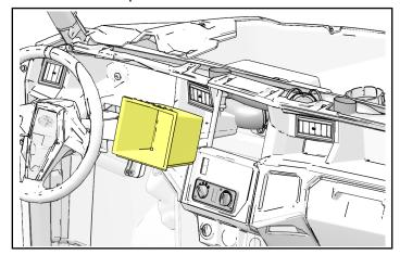
j. Carefully connect instrument cluster electrical harness, then reinstall instrument cluster using retained hex head screws ©.
