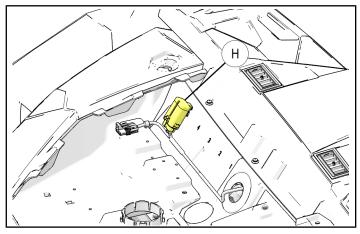
c. Route main heater harness switch panel connectors rearward towards center control panel.
