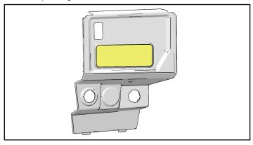
b. Orient switch panel **(6)** so blower control is on LH side and temperature control is on RH side, then install into opening until tabs lock in place.
