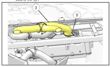
d. Duct 4: Route from heater core to RH outboard dash and RH defrost. Secure duct at heater core with cable tie 5.
