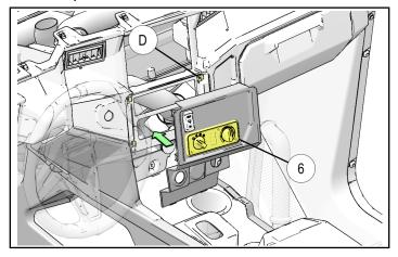
Reinstall center storage box by hooking lower edge of box in dash opening, then tip upper edge of box into dash until locking tabs snap into dash panel.
