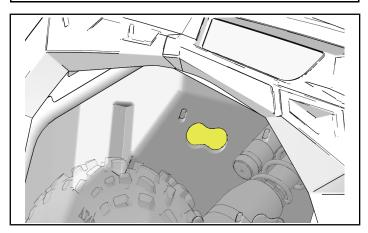
b. Drill three 5/16 inch (8 mm) holes in firewall for heater core mounting screws ②.
