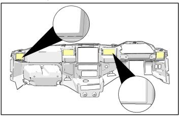
c. CENTER CONSOLE SIDE PANELS (LH and RH): Using 2-1/2 inch (64 mm) hole saw, cut hole at center of recessed markings.
