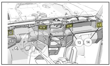
f. Carefully reconnect electrical harnesses and lower interior lights, then reinstall main dash panel using retained fasteners: four push pin rivets (£) and six screws (£). Reference Step 3d.
