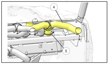
e. Lift main dash panel into position, carefully pulling ducts ②, ③, and ④ through corresponding dash vent openings. Use cable ties ⑤ to secure outboard ducts to square vents ⑭ and inboard ducts to rectangular vents ⑤. Snap vents into openings.
