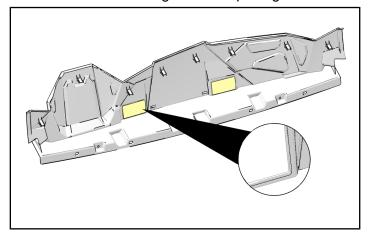
MAIN DASH PANEL: Cut two rectangular vent openings and two square vent openings along INSIDE EDGE of recessed markings. Debur openings.
