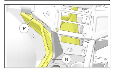
vi. Remove main dash panel, carefully disconnecting electrical harnesses and three lower interior lights ©.
