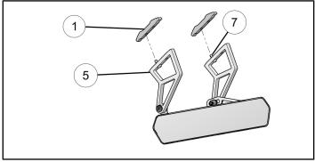
4. Rotate clamps ① so mirror assembly can be inserted up through slot in vehicle mount plate, then rotate clamps ① back so remaining screws ⑦ can be installed as shown.
