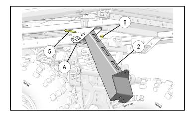
Swing back end of LH support ② up and loosely install to tailgate support structure using one screw
