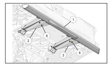
6. Torque Step 2 fasteners (5) (6) and Step 3 fasteners (4) (6) to specification.
