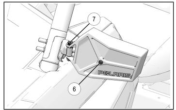
b. Fine mirror adjustment (rotation and tilt) achieved by loosening screw (6) as shown, adjusting mirror, then tightening screw. Do not overtighten screw.
