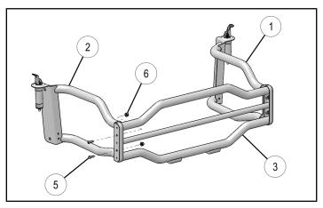
4. Lower assembled bed extender into vehicle until expansion anchors (a) are fully seated, then depress upper cams to lock in place. If installation is loose, remove extender assembly from vehicle, tighten nuts at base of expansion anchors, and reinstall.
