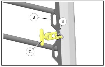
4. Install shoulder screw ③ to fixed rack ④. Tighten screw. Repeat for RH side.
