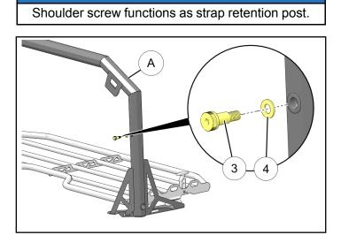
3. Raise moveable rack (B), then secure two straps (C) to shoulder screws (3) installed in previous step.
