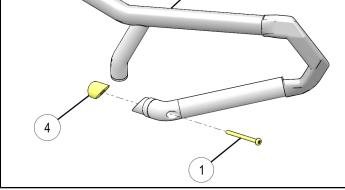
4. Fully insert threaded mount ④ and tapered end of LH bumper ③ into existing bumper ④.
