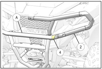
5. Loosely install screw (6) up through mounting ears in existing bumper (A), then into LH bumper (2).
