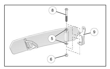
Assemble clamps ② and ③ to mirror using screw ④, washers ⑤, and nut ⑥ as shown in Kit Contents. Repeat for opposite end of mirror. Do not tighten fasteners at this time.
