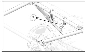
4. Place mirror in desired position and tighten all fasteners. Torque to specification.
