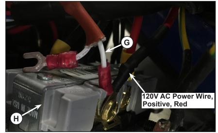
Connect the other lead (J) from the Cold Weather kit wire connector to the 120V, AC receptacle (H), negative side, from the back of the generator set front control panel.
