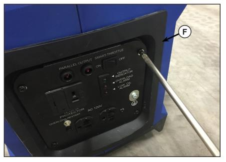
7. Remove the generator front control panel (F) with Phillips screw driver.
