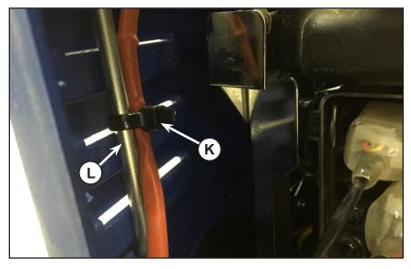
Route the Cold Weather kit harness by using cable zip ties (K) to connect to the stainless steel support rod (L).
