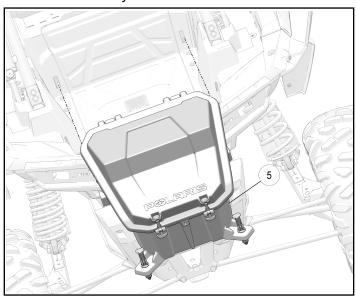
5. Install the storage box base ⑤ onto the vehicle body.
