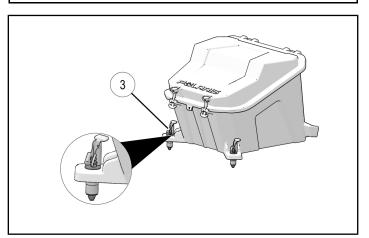
4. Slide the box on the vehicle so that storage box base ⑤ protrusions on the box are seated into the slot on the body.
