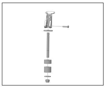
3. Install lock and ride anchors 3 on to the cargo box.
