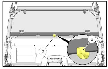
b. Drill 1/4 inch (6 mm) hole through close-off extension panel ② at marked location.
