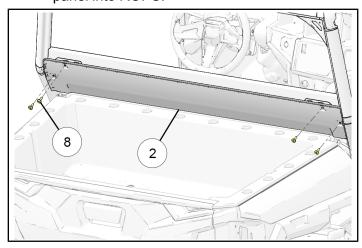
c. Using extension panel ② as template, mark five holes in existing vehicle close-off panel.
