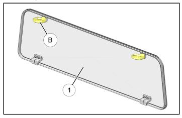
b. Install rear panel ① by inserting two lower brackets ② into ROPS cross-member. Pivot panel forward into ROPS, then rotate handles
