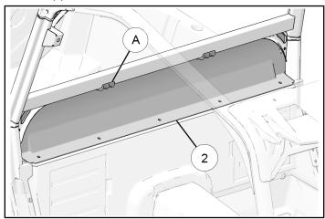
b. Pivot extension panel ② forward into ROPS, then loosely install four screws ⑧ through panel into ROPS.
