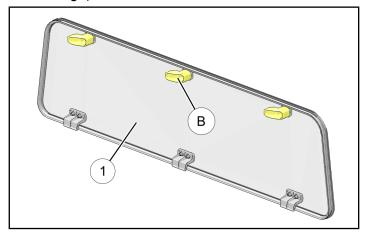
b. Install rear panel ① by inserting three lower brackets ② into ROPS cross-member. Pivot panel forward into ROPS, then rotate handles
