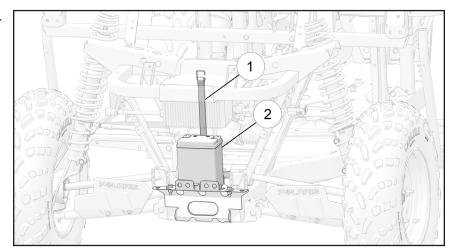
Reroute the wires as shown in figure below. Connect the positive and negative cables to the respective battery terminals.
