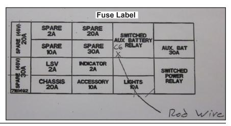
13. Cut the red wire (J). Strip the fuse block side and apply electrical tape to the harness side.
