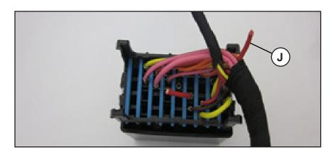
14. Slide the barrel splice and yellow wire (K) onto the stripped fuse block wire. Crimp and apply heat shrink to the exposed conductor.
