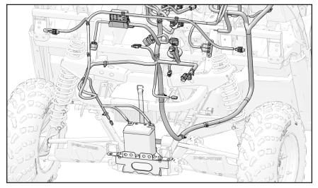
**NOTE:** To avoid overcharging the 12V batteries, this charging system only functions when the vehicle key is in the "ON" position. The 12V battery kit will recharge from the drive system batteries while you are driving the vehicle. To prevent possible accidents and injuries, Polaris strongly recommends against leaving the vehicle key in the "ON" position while recharging the vehicle's drive system batteries.
