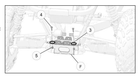
7. Place the battery (2) on the mounting bracket (3).
