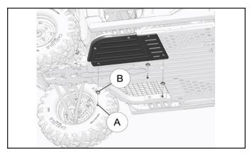
Fasten two M6 screws (3) and washers (4) as shown in figure.
