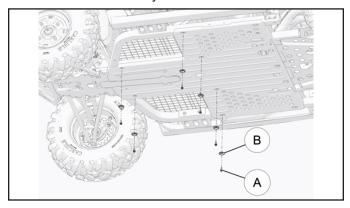
3. Align left hand side skid plate (1) with holes of existing skid plate as shown in figure.
