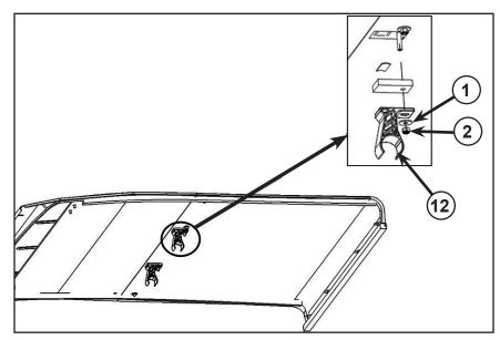
4. Place the roof on the top of the vehicle. See figure.
