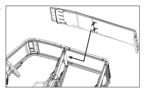
5. Push the center supports on cab frame tube (C), so that these can be fit onto the tube. See figure.
