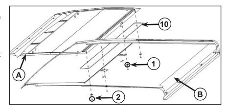
3. Attach two clamps (12) to the steel roof assembly as shown and secure it by tightening M8 nut (2) and relevant washer (1).
