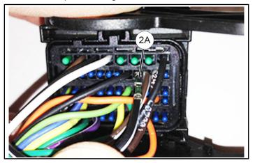
g. Reinsert purple TPA clip (F) into connector, ensuring clip fully seats in connector.
