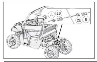
5. Route terminal pin 2A on reverse beeper harness② forward along main chassis harness.
