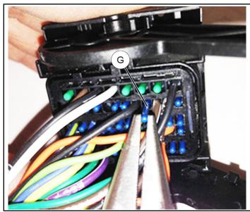
f. Insert terminal pin 2A into cavity 45. Pin should easily slide in and "click" into place. If not, rotate pin 180 degrees and reinsert.
