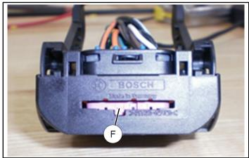
h. Reinstall back cover E to ECU connector until it locks into place.
