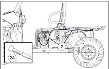
6. Install terminal pin 2A to ECU connector.
