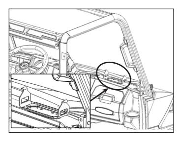
2. Before installing audio mount base (6), place and allign the pad (9) with holes on dashboard and audio mount as shown in figure.
