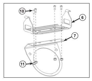
6. Align and Install audio mount bracket assembly on the pod using two tuflok rivets (12) as shown in figure.
