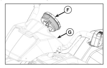
3. If you cannot remove the cluster by hand, consider removing the upper pod (G) by removing three screws (H) allowing access to push the cluster out from the back side of the assembly as shown in figure.
