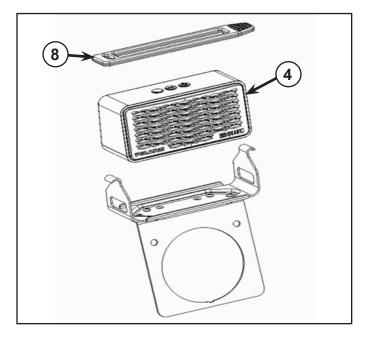
6. Align and Install audio mount assembly using two tuflok rivets (L) as shown in figure.
