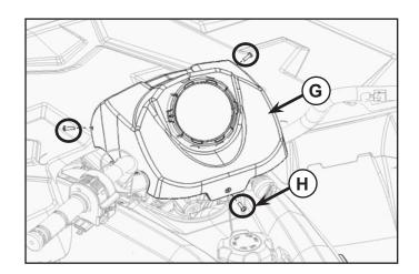
4. Align audio mount bracket (7) with pod (G) and use as template to drill the holes of dia 5/16" as shown in figure.
