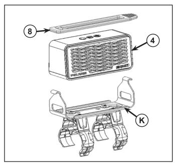
3. Snap fit bluetooth speaker assembly on to the ROPS tube (1.75" Dia) at any required location.
