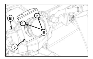
4. Fasten audio mount bracket (5) with audio mount base (6) using four screws (10) and nyloc nuts (11). Tighten screws until snug.
