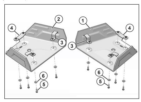
3. Adjust and install Rear A-Arm guards on the A-Arms as shown in figure.
