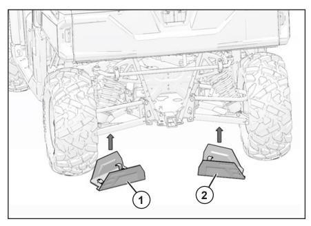
4. Tighten the M6 screws to torque 8 ft. lbs. (10.8 Nm) as shown in figure.
