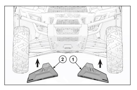
5. Tighten the M6 screws to torque 8 ft. lbs. (10.8 Nm).
