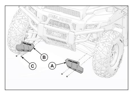
3. Loosely install the clamps (3) on the front A-arm guards, LH (1) and RH (2) using M6 screws (4) and washers (5) as shown in figure.
