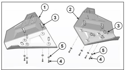
4. Adjust and install LH (1) and RH (2) A-Arm guards on the A-Arms as shown in figure.
