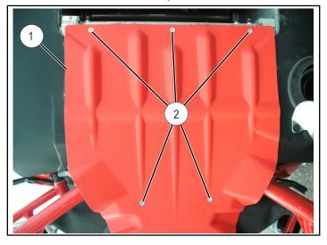
7. Extreme skid plate: Install two self-drilling screws
