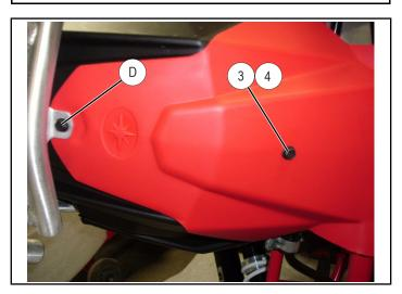
6. Ultimate skid plate: Install five self-drilling screws
